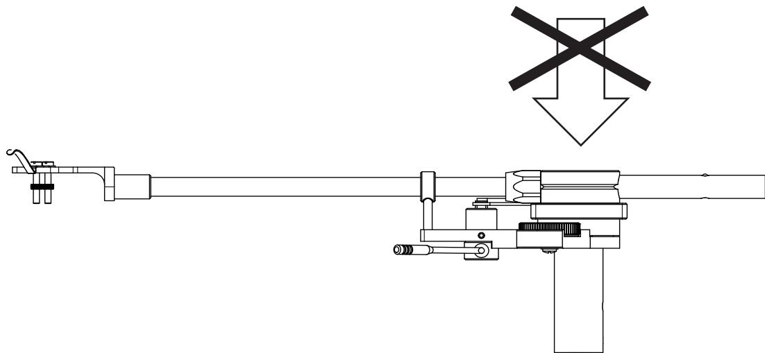
The plastic transport spacer protects the flexure bearing. Remove it once the tonearm is mounted on the turntable. There is no need to use the spacer in day to day operation of the tonearm. Please understand that the spacer cannot completely prevent damage from mishandling.
